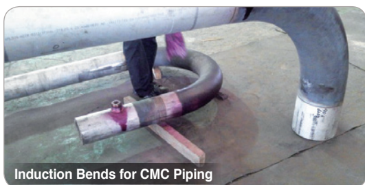
Welded Induction Bend Spools. TP304L
