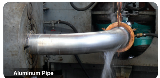
Induction bends applied to Amonia & Urea plant pipings
