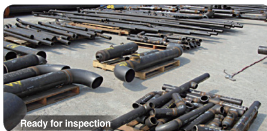
Welding Prefabrication of Process Piping, TP316L
