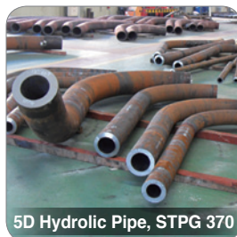
Induction bends applied to Amonia & Urea plant pipings
